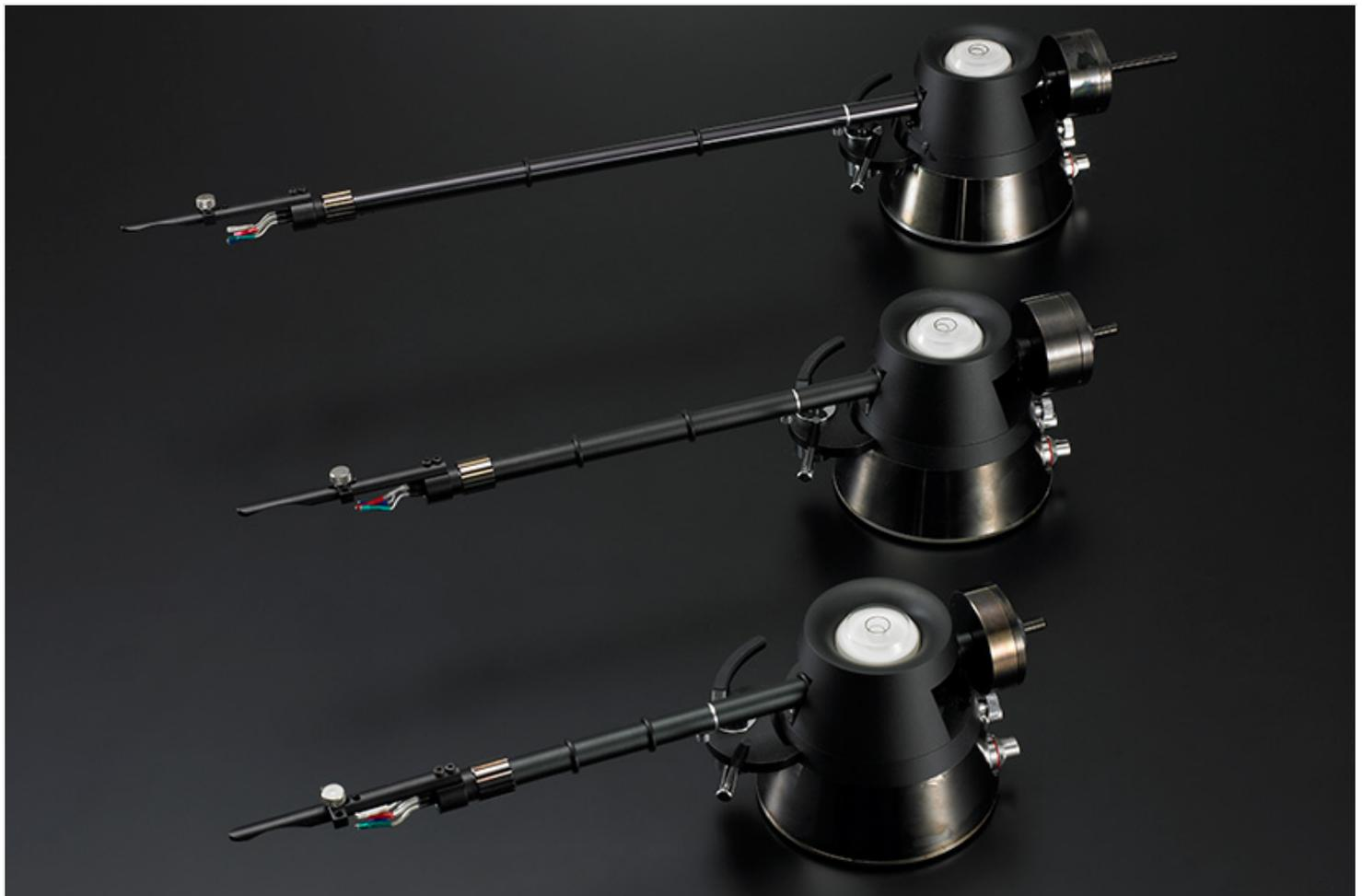
The armtube itself is fairly small in diameter and appears to be aluminium, it has a collet for the detachable headshell and two 'O' rings along it presumably for damping purposes. The headshell is rather unusual too albeit not dissimilar to one created by the Funk Firm a few years back, it consists of an aluminium protrusion with three holes in it and a separate
