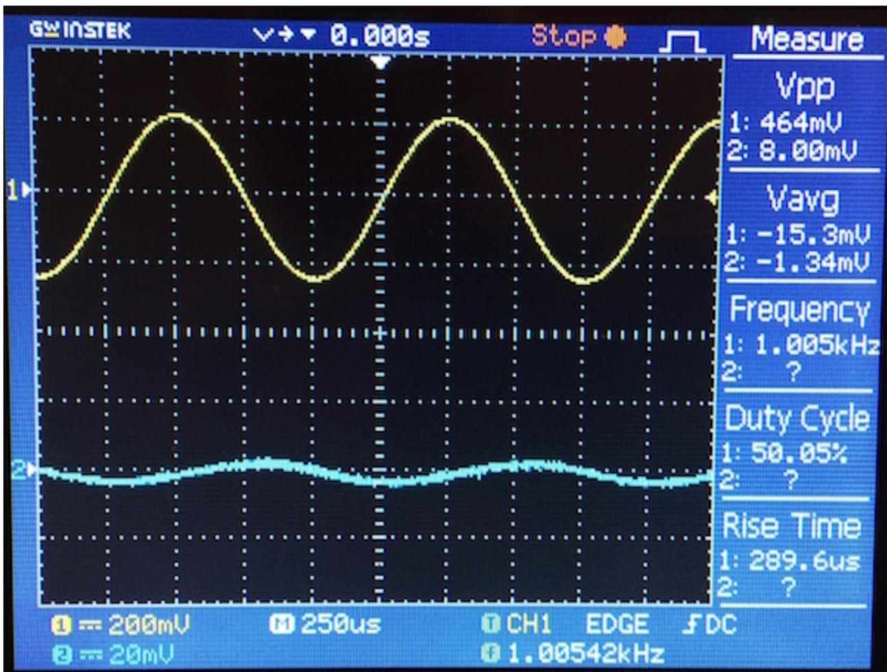
The oscilloscope trace on top in yellow shows the 1kHz test tone modulating the left channel of the test record. Theoretically the blue trace should be flat, which would mean no crosstalk but of course there's always some. In this case the blue line is about as flat as I've seen. Usually there's more of a visible wave, indicating higher crosstalk.
