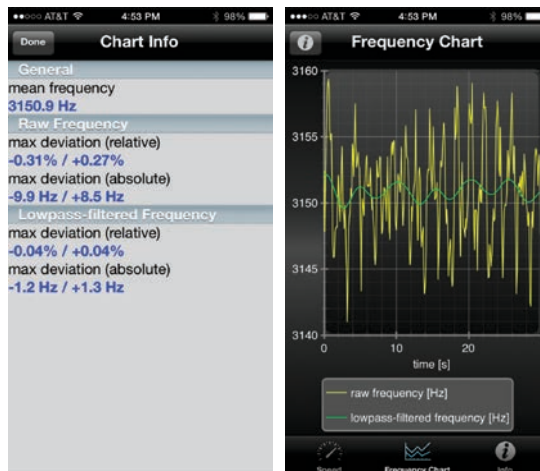
Fig.1 (near right) Brinkmann Spyder, speed measurements from Dr. Feickert iPhone app.
