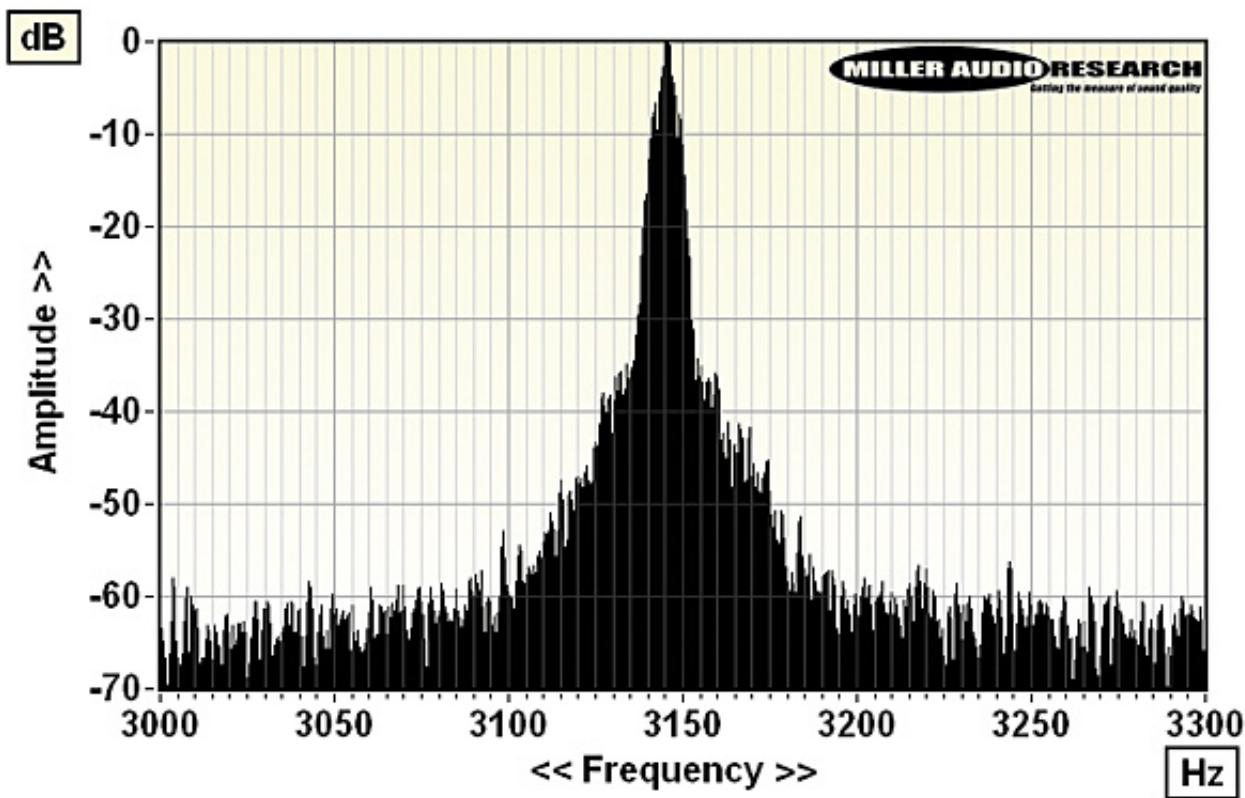
Wow and flutter re. 3150Hz tone at 5cm/sec (plotted  $\pm 150\text{Hz}$ , 5Hz per
