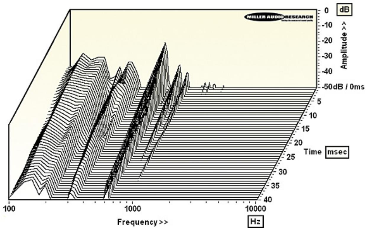
Cumulative tonearm resonant decay spectrum, illustrating various bearing, pillar and ‘tube’ vibration modes spanning 100Hz-10kHz over 40msec
