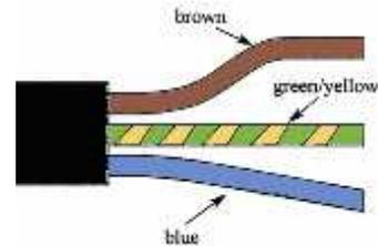
For safety reasons, the equipment must be provided with an earth connection.
