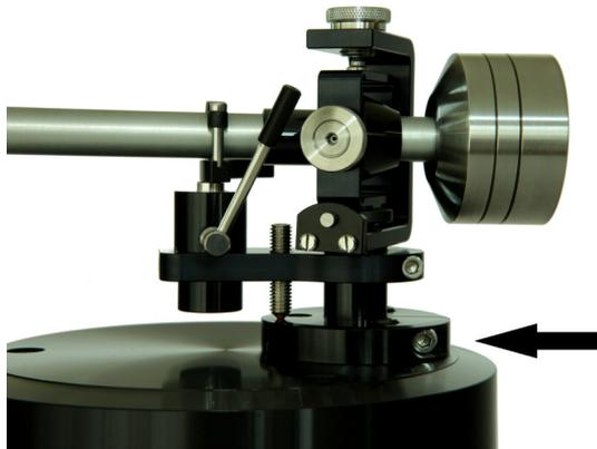
Now adjust the vertical tracking angle (VTA). It's usually best to start with the tonearm tube parallel to the LP when the tonearm is lowered onto the record surface. (Proper Stylus force must be applied before obtaining parallel adjustment.) This usually is close to proper VTA and provides a good reference point.
